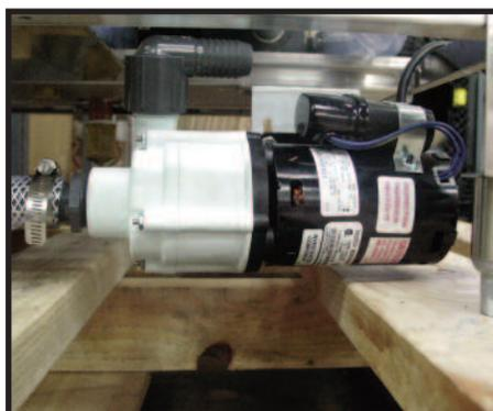
**Pump-Out Drain** is available for restricted or upward drainage requirements.
